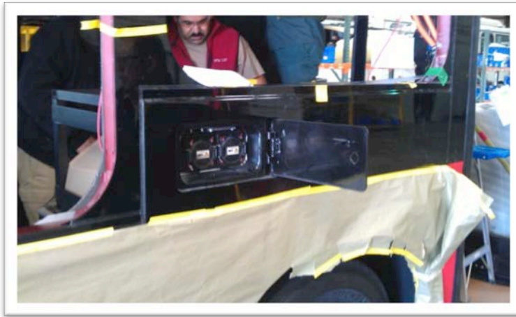
Figure 3.16 New Location of BYD Bus Charger Receptacle - Front Right of Bus
